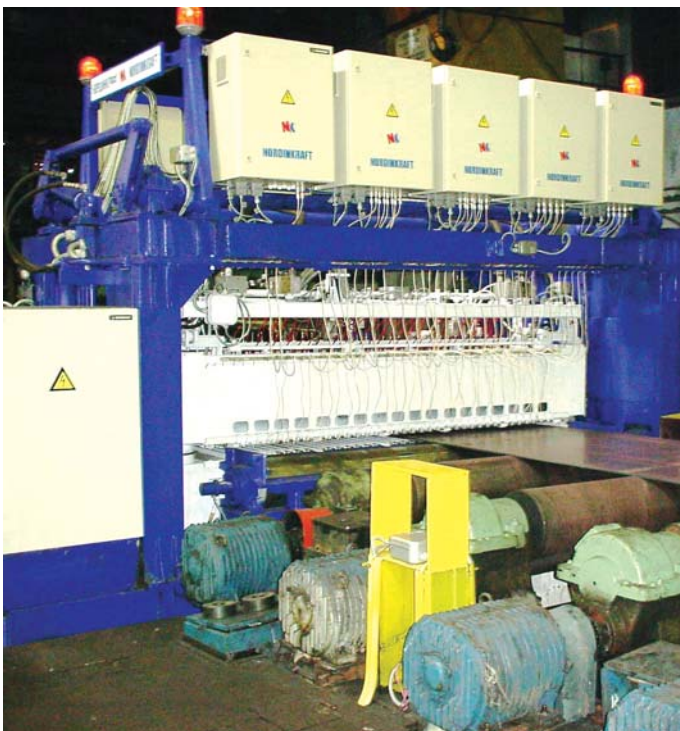
Pic. 9. Plate testing system "Sever-6-08-2800", JSC "Magnitogorsk Iron and Steel Works" (2001).
