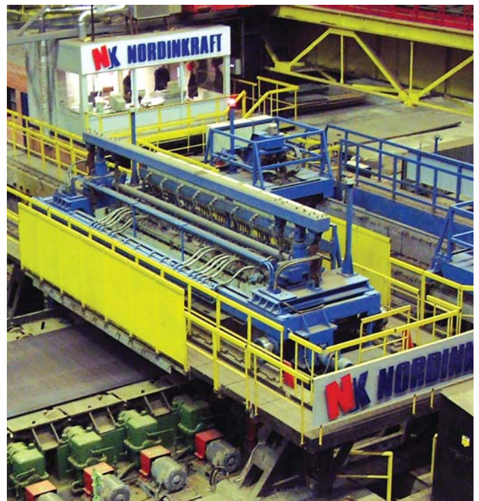
Pic. 10. Plate testing system "Sever 6-08-5000-HT" – Plate rolling shop-3, JSC "Severstal", Kolpino (2003).
