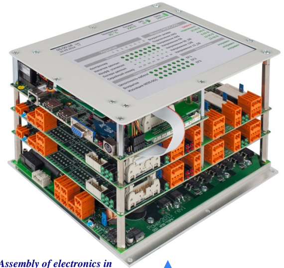
Assembly of electronics in standard PC-104 for demanding use
