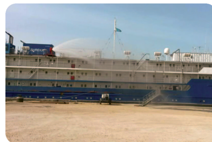
Fire monitors on “Shkotov”-, “Princessa Caspia”-ships Kazakhstan
